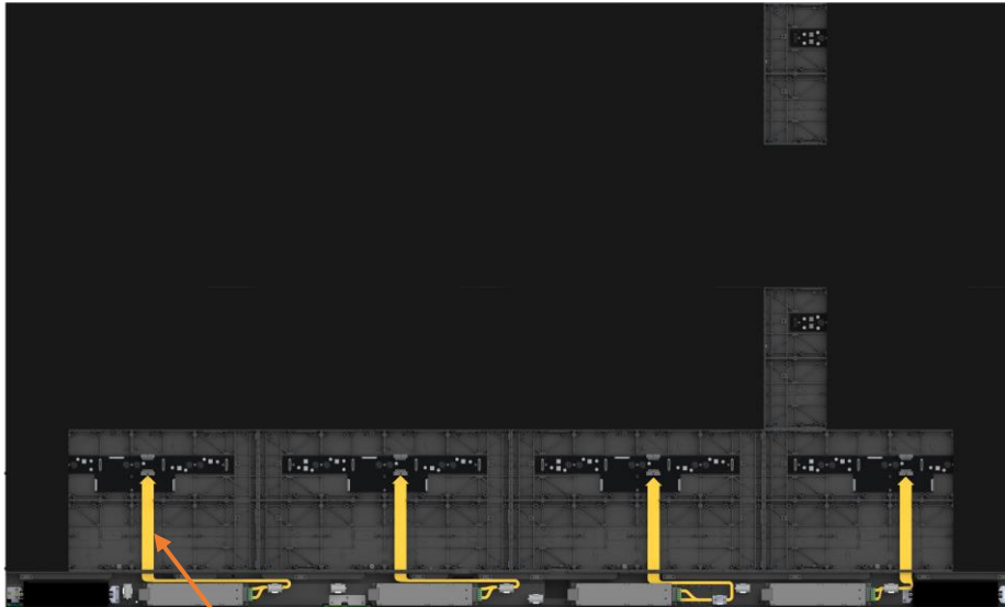
4X Column Power Cables
