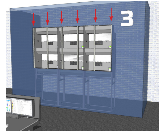
Step 3 - Installation of the substructure for the LED video wall on the cube housings
