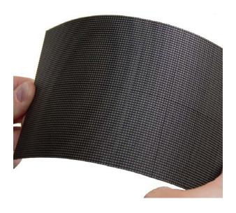
Leyard Europe CarbonLight<sup>™</sup> CLI Flex<sup>™</sup> Series pliable LED video wall displays combine to create immersive and eye-catching concave or convex curved video walls. The LED modules are literally bendable, ideal for smoothly curved walls, waves, halos or column wraps. The modules can form curves as tight as 25" or 637mm without colour shift, offering a more visually-appealing alternative to faceting flat LED cabinets into segmented curves.
